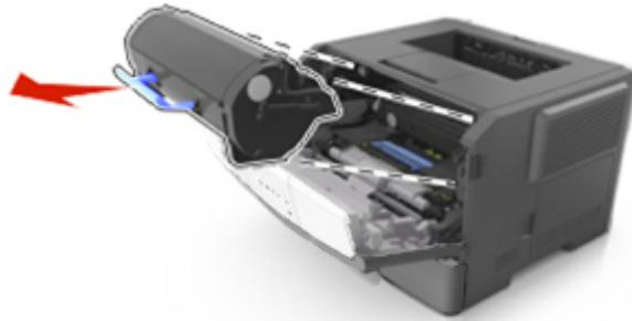
3. Lift the blue handle, and then pull the imaging unit out of the printer.
